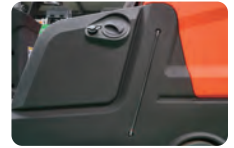
Water injection port and water level indicator Display clear water tank water level, large opening water injection port, easy to add clear water.
